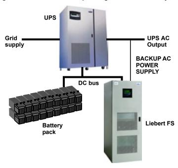
Figure 157 Multiple Liebert FS+DC units operating with a UPS in conjunction with batteries
